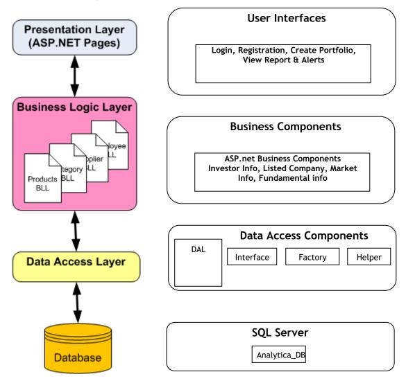
**Figure-4: System Architecture**
