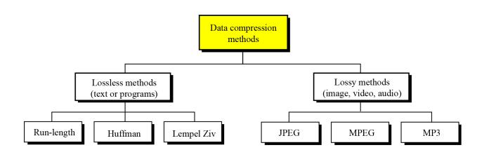
Figure 2. 2 Typical Data Compression Techniques
