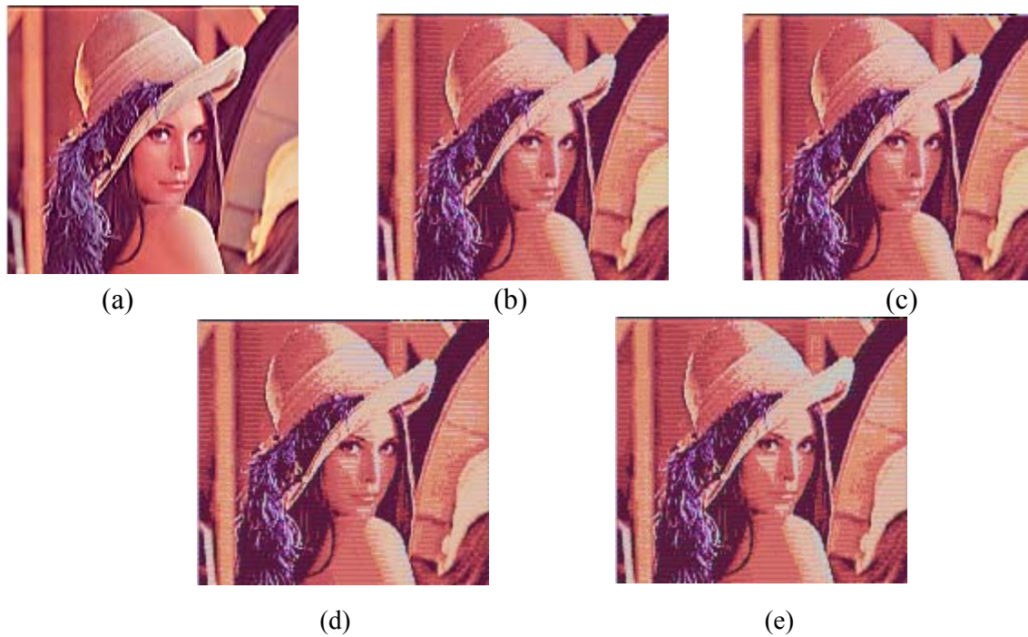
Figure 8: Showing the quality of the image after compressing the standard “Lena” image in (a). (b), (c), (d) and (e) are the images having 256, 128,64 and 32 colors respectively.
